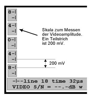
The video level of the fed-in RF signal can also be measured in the SCOPE menu.
